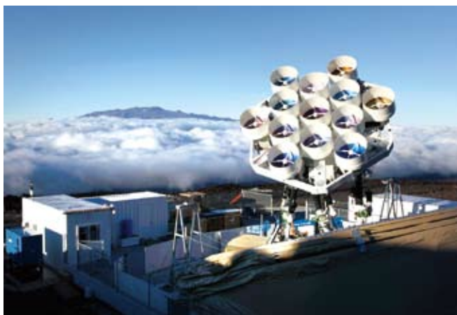
AMiBA was upgraded from its 7-element 0.6m reflector configuration to its new 13-element 1.2m reflector configuration during 2009, and resumed operations on Mauna Loa in Hawaii.
