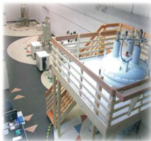
↑ The High-field Nuclear Magnetic Resonance Center at Academia Sinica was commissioned to support structural genomic and drug development studies. It currently houses several state-of-the-art NMR spectrometers, including one at 800 MHz (front), three at 600 MHz, and one at 500 MHz.
